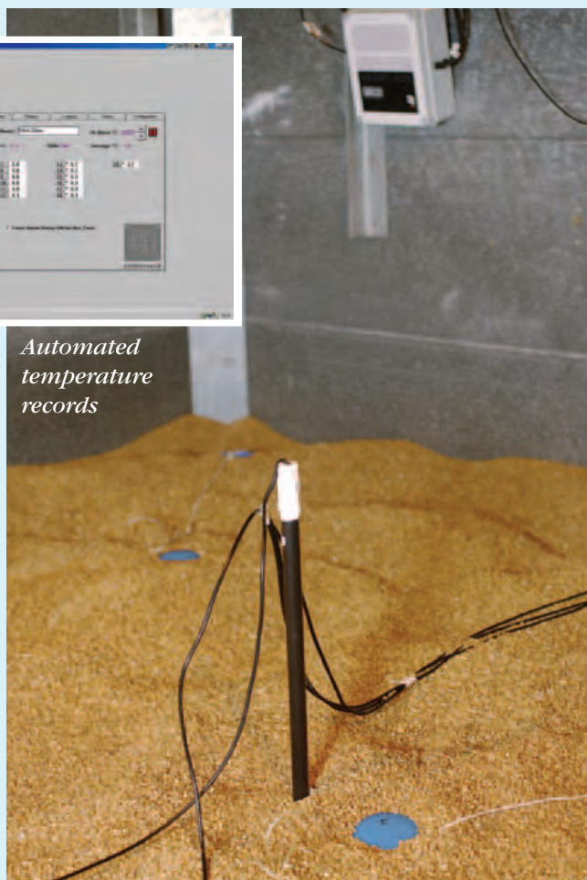
Permanent probe arrays can be linked to record keeping software to identify potential problems.
