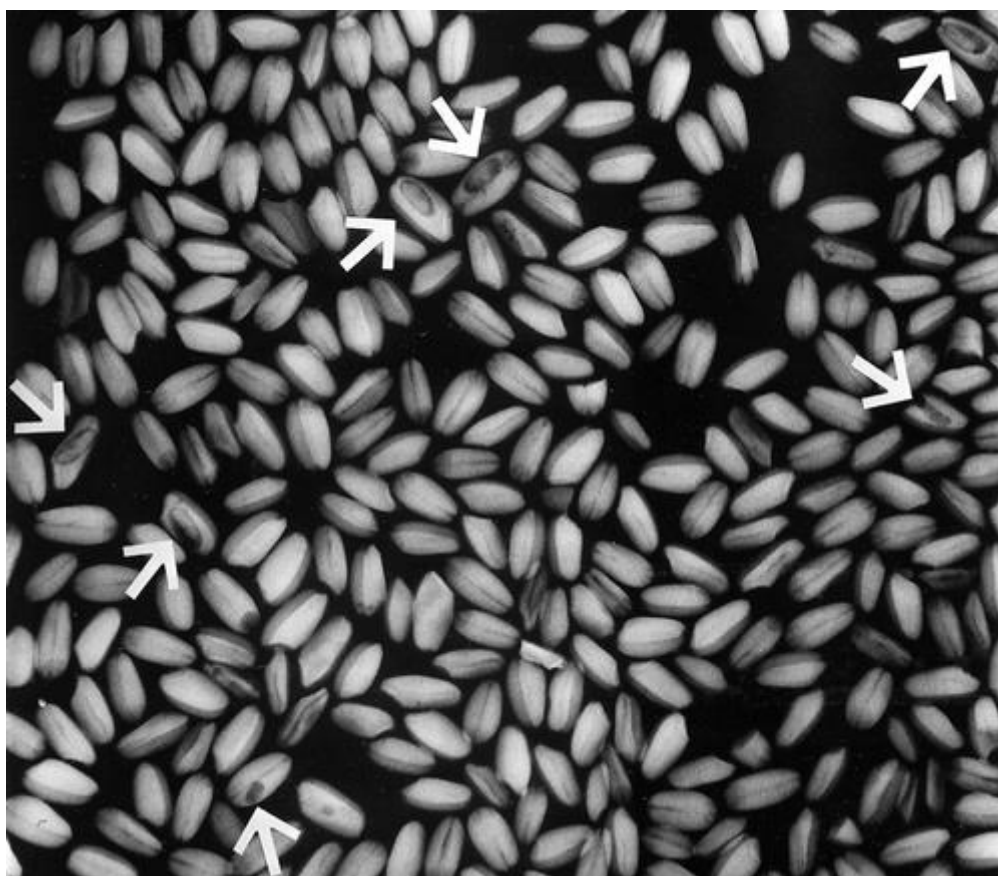
Fig. 7.10. X-ray of wheat, showing internal infestation (arrows). (Courtesy J. Pederson)
