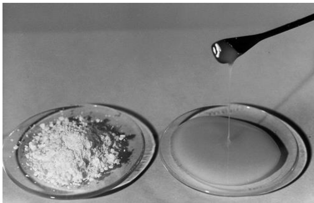
Fig. 13.8. Starch-water mixture (1:1, left) and starch-water-sugar mixture (1:1:1, right). (Reprinted, with permission, from Ghiasi et al 1982)
