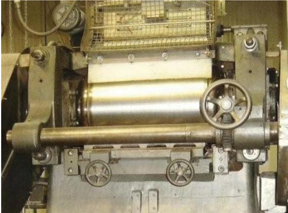
Fig. 15.2. A photograph of a set of flaking rolls. (Courtesy D. Ortiz, Kellogg Company, Battle Creek, MI)
