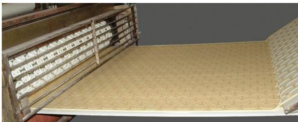
Fig. 13.4. Photograph showing continuous production of cookie dough pieces by rotary cutting of a dough sheet. The dough scrap is removed by lifting it away. (Courtesy D. Ortiz, Kellogg Company, Battle Creek, MI)
