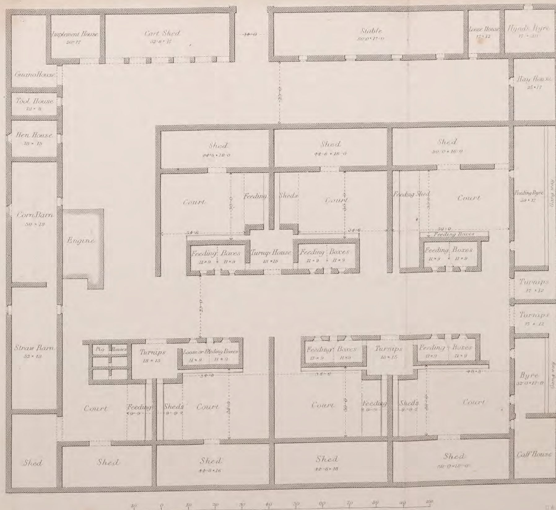
PLAN OF HOMESTEAD FOR A FARM OF 600 ACRES BY M R . R. HARDIE.
