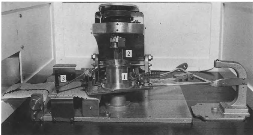
Figure 8.3. Micro-mixograph of Swanson and Working for the analysis of dough characteristics; the kneading system has been tilted; kneading basin (1), kneading pens (2) and recorder (3).
